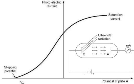
Some of the photoelectrons that emerge from the metal surface have enough energy to reach the cathode despite its negative polarity, and they constitute the measured current. As long as the voltage is increased to a higher negative voltage,  $V_0$ , no more photoelectrons achieve, as indicated by current dropping to zero. This potential is known as stopping potential.
