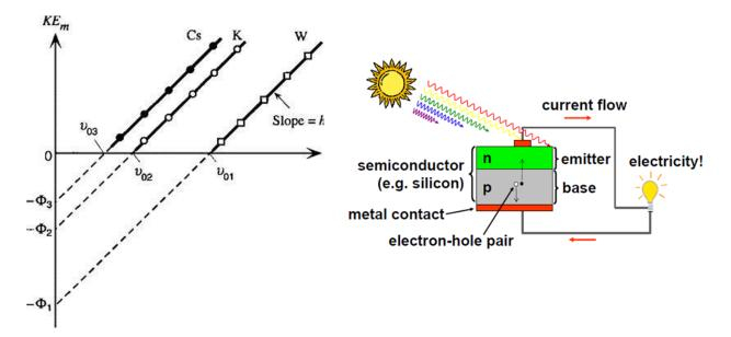
**Solar** (or photovoltaic) **cells** convert the sun's energy into electricity. Whether they're adorning your calculator or orbiting our planet on satellites, they rely on the **photoelectric effect**: the ability of matter to emit electrons when a light is shone on it.
