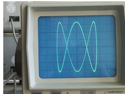
Lissajous figures on oscilloscope
