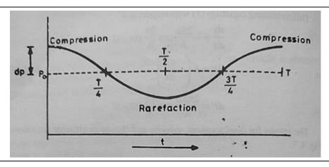
This is a graph representing change in pressure with respect to time. Here,  $P_o$  is the normal pressure which the medium possesses in the absence of the propagation of wave.
