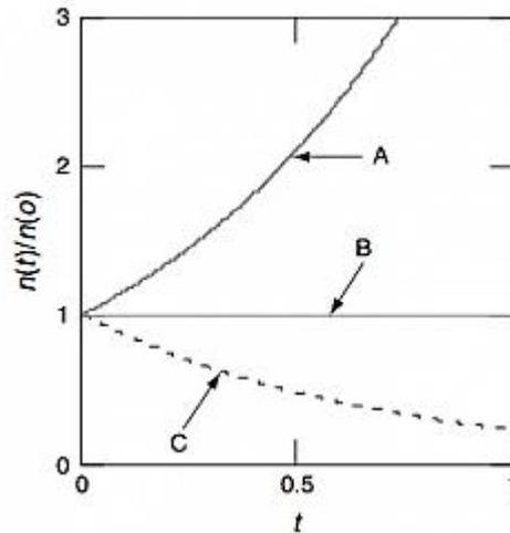
Reactor criticality. A – supercritical state; B – critical state; C – subcritical state
