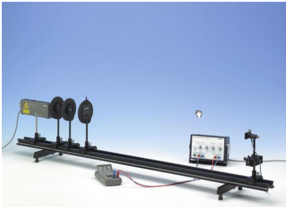
Fig.1 Experimental set-up for the investigation of the diffraction intensity due to double slit.
